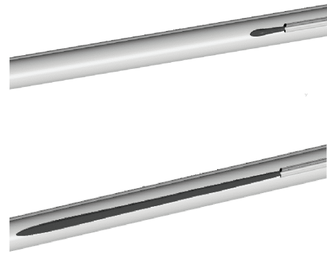
Figure 12: Emerging bolus of injectant from a catheter, an example of computational results.
